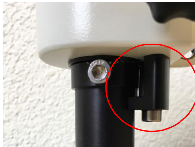
Figure 3: Detailed view of the retention fixture as an additional means of securing the M220 Optics Carrier
